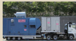
Instillation of emergency air-cooled generators
