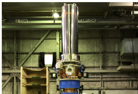
Joint research on gyrotron, plasma heating system
