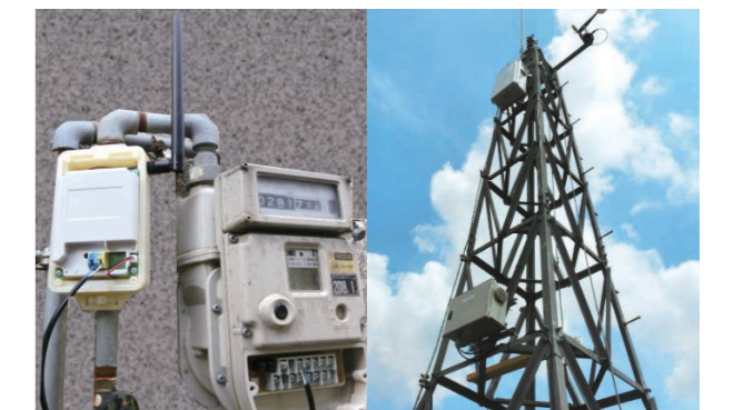
Wireless device and base station for automatic LP gas detection
