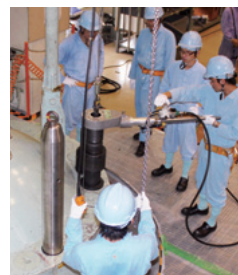
Practicing a major inspection on a nuclear reactor using a mock-up of a reactor vessel
