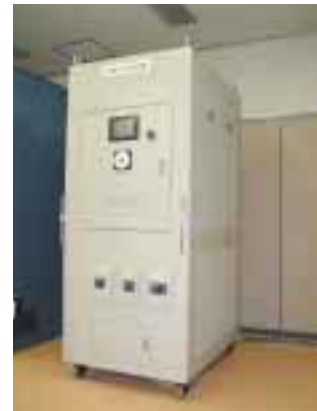
12-kVA SiC 3-phase inverter equipment
