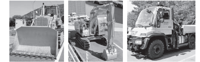
Dozer shovel for debris removal, Power shovel for debris removal, Large truck with crane ideal for work in hard-to-reach places
