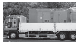
Power supply vehicles
