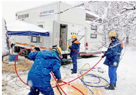
Emergency power transmission with a high-voltage generator vehicle
