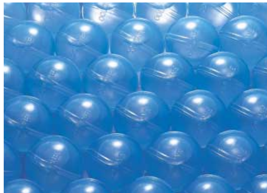
Resin balls. Compact heat-storage material for home use.
