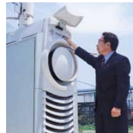
Micro gas turbine undergoing field test.
