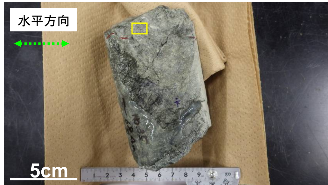
No. 35 68.40mの断層面(下盤上面)
