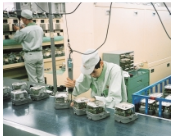
Checking and repairing wattmeters for reuse (Kansai Keiki Kogyo, Inc.)
