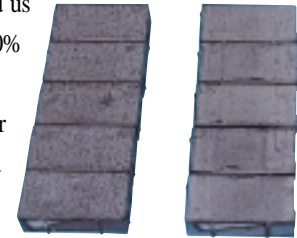
Oxidized baked bricks containing coal ash
