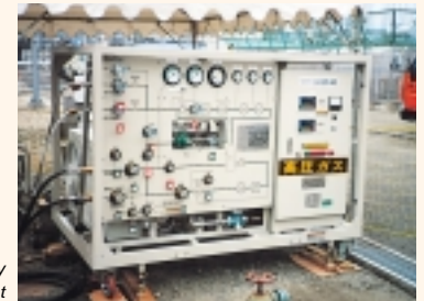
SF 6 gas recovery equipment
