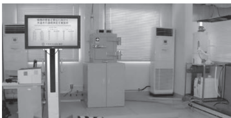
Automatically detects presence of radioactive substances and displays results on a monitor.
