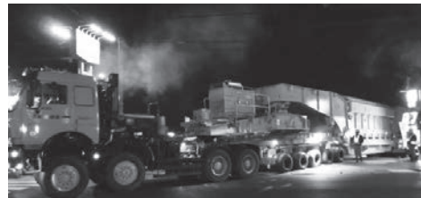
Hauling the transformer by special truck trailer setup
