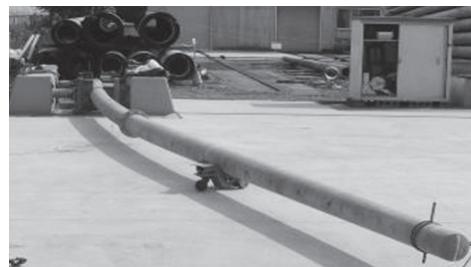
Bending failure test performed on a dismantled concrete utility pole
