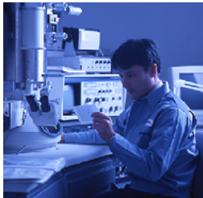
Metal fatigue inspection by electron microscope
